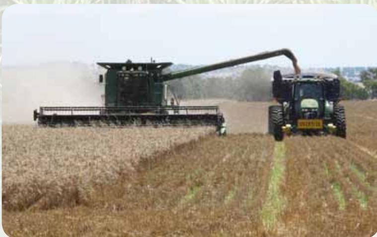
**Matching additional machinery:** An auger extension on this header in a 9-metre CTF system means the tractor and chaser bin are able to stay on the tracks during loading.
