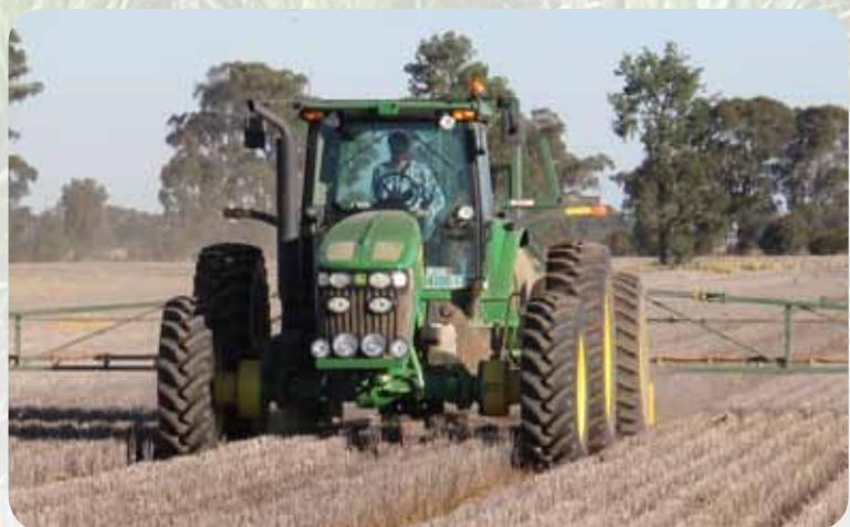
**Matching axle widths:** The front axle of this spraying tractor was extended with factory fitted cotton reel spacers and a three metre axle made for the boomspray to suit permanent three-metre tracks.
