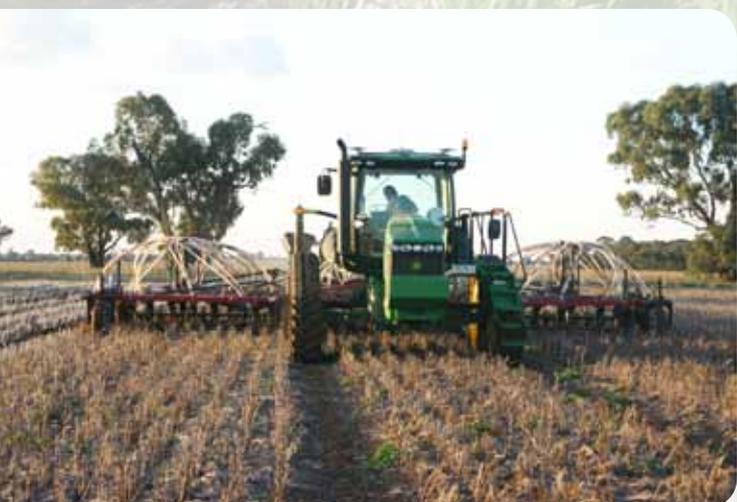
A John Deere track tractor was purchased in 2011, with accurate steering making it ideal for inter-row sowing. Better traction means it will also be used for spraying/spreading in wet conditions.
