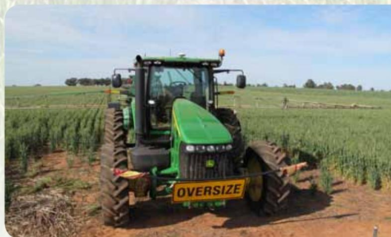
**Power requirements:** Controlling wheel traffic to permanent tracks has meant this lower horsepower tractor can now be used for all operations (sowing, spraying, spreading and chaser bin).
